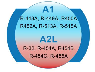
State and Federal regulations are now in place to phase down/phase out the use of high GWP HFC refrigerants. These regulations will impact new systems, on going service and retrofits. This class will introduce you to the next generation of A1 - A2L & Natural Refrigerants and their adoption in AC, Heat Pumps, Chillers, and Refrigeration.
